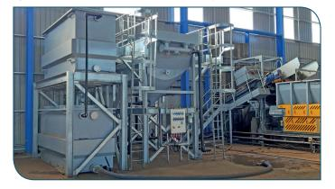
SPS developed a bespoke solution, including a Lamella Clairfier HB40R, which has the built-in mechanism to be raised, eliminating the need for any water to be pumped, saving significantly on costs. The system is highly effective, removing around 80% of all suspended solids in the wastewater; all while processing 15m3 of water per hour.
