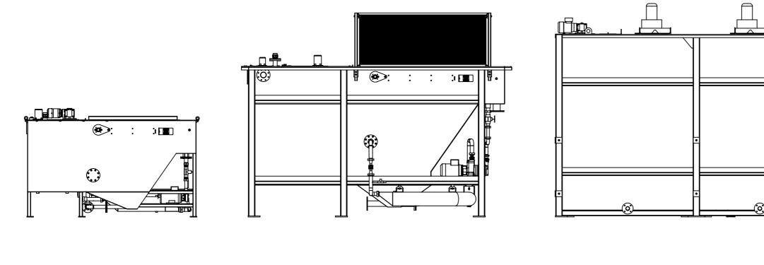
**iD5** L: 2597mm W: 1210mm H: 1614mm **iD10** L: 4048mm W: 1715mm H: 3054mm H: 2250 (BRIM) **iD25** L: 7157mm W: 1880mm H: 2732mm H: (BRIM)
