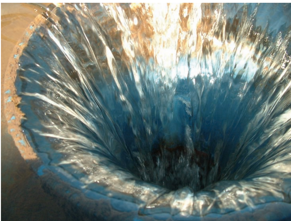
Treated water discharging out of a Siltbuster clarifier.
